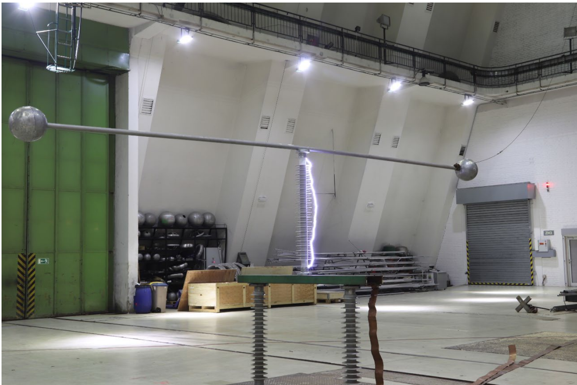
Figure 4 Test arrangement during the critical impulse flashover tests
