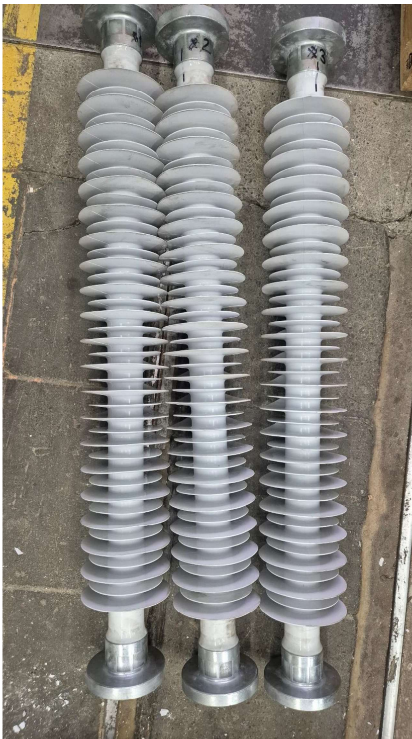
Photo 4 – Samples after the torsional test
