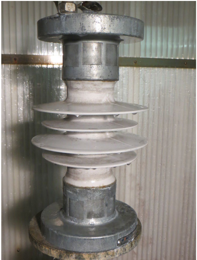
Figure 17 Test sample in vertical test position, before and after tracking end erosion test – 1000h salt fog test
