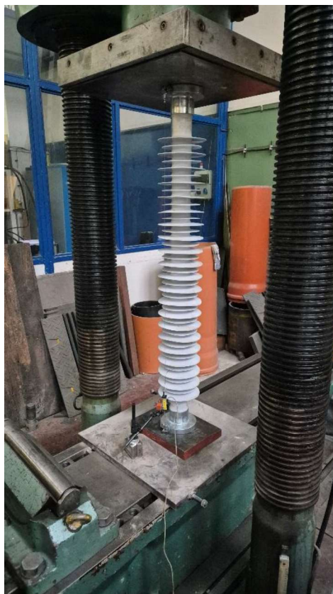
Photo 1 – Characteristic arrangement of the compression test
