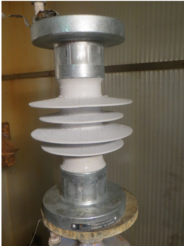
Figure 17 Test sample in vertical test position, before and after tracking end erosion test – 1000h salt fog test
