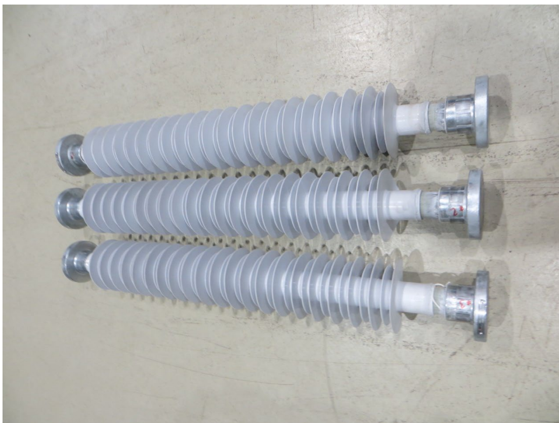
Figure 16 Test samples after tensile load test
