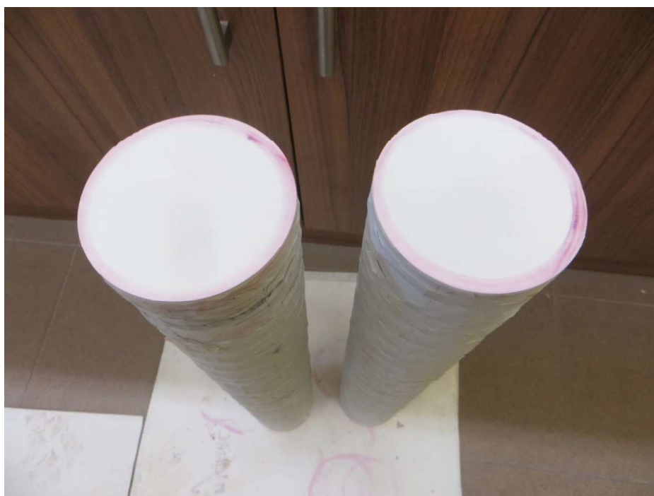
Photo 2: View of sample after the dye penetration test
