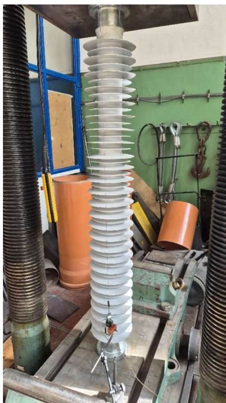
Photo 1 – Characteristic arrangement of the compression test
